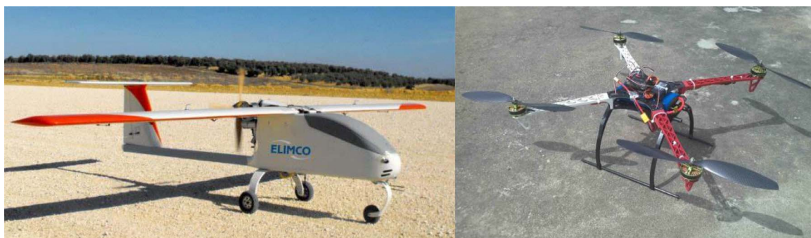
a) E500 fixed-wing UAV by ELIMCO (©ELIMCO SOLUCIONES INTEGRALES S.A.) b) Rotary-wing UAV used by ACE-TI research group (University of Seville)
