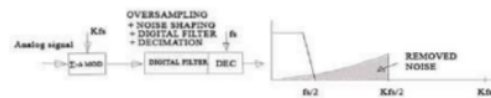
Figure C. Noise shaping is employed to push most of the noise spectrum to higher frequency so that the in-band noise is reduced significantly.
