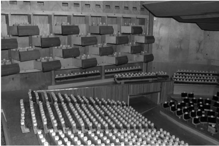
Figure 8.5 Physical model: acoustic model of a concert hall (© Kirkegaard Associates)
