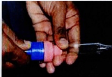
Figure 10(e): 1 To load the silicone syringe, remove the plunger and fill the barrel of the syringe with the thoroughly mixed material
