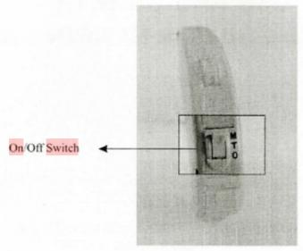
The On/Off switch is used to turn the hearing aid on, set it on 'T' mode, or to turn the hearing aid off. This helps in preventing battery drainage when the hearing aid is not in use. In some hearing aids, the battery compartment itself acts as an On/Off switch.
