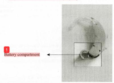
While inserting the battery into the battery compartment, check that the positive end of the battery (marked with +) is in contact with the positive end of the battery compartment (also marked with +), and the negative end of the battery (-) is in contact with the negative end of the battery compartment (-).
