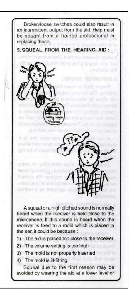
on the opposite side (if used on one side). If this is not the cause for a squeal, check the volume control setting, bring it down if it is too high. Too high a volume will also over-amplify the sound which the wearer may not be able to tolerate. This would also distort the speech heard through the aid. If reduction in volume does not stop the squeal, check the mold.
