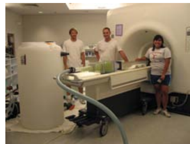
Figure 1. Chris Elkins, PhD, Mike Benson, PhD, and Sayuri Yapa, MS, researchers from Mechanical Engineering prepare for MR scans using a mechanical flow phantom at the 1.5T whole body magnet.
