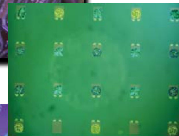
Image 3: The image below results from work in the CCNE program, which is developing magnetic-nanoparticle detecting sensors to improve cancer diagnosis. Each of the tiny squares in the above image is a sensor (Sebastian J. Osterfeld, PhD and Shan X. Wang, PhD).
