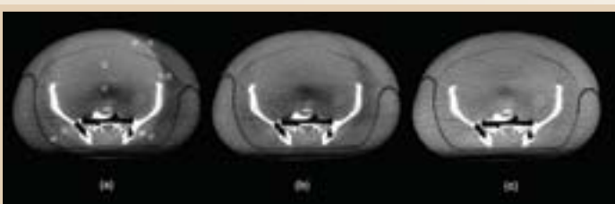
CT reconstructions for three cases. (a) No lag correction with an average error of 43 HU, (b) an LTI correction from the optimal exposure with 17 HU error, and (c) the non-LTI correction with 11 HU average ROI error.
