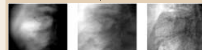
SBDX system DTS images focused on a lung nodule when the anthropomorphic phantom is located at (left) y=100cm (larger tomographic angle) and (middle) y=50cm. (right) Projection image with the lung nodule centered. Window and level have been adjusted (for all images) to maximize lung nodule visualization.
