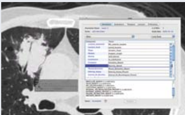
IPAD 1 Use of our iPAD tool to annotate a lung tumor on a CT scan. In addition to the controlled terminology selected using the interface, computer algorithms will characterize image features within the region of interest.
