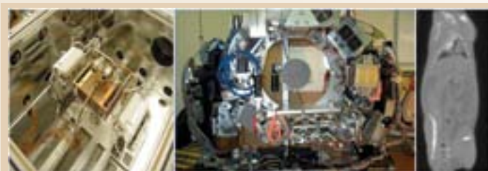
(left) photograph of the 2x4 module in its vacuum vessel (center) IGCT gantry (right) sagittal rat image
