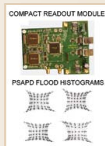
Top, the compact readout electronics module. Bottom, collected data demonstrates readout capability through the individual crystal separation in the flood histograms.
