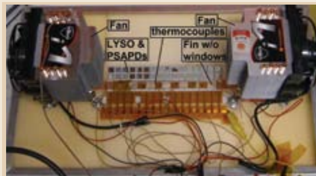
Experimental device for temperature measurement using fin without windows to cool PSAPDs
