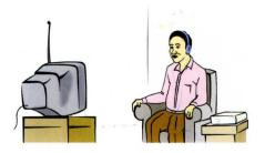
TV. The amplifier sends the sound to a headset through the wire. The major disadvantage of this system is that the wire is not too long, and the listener has to stay close to the television. Moreover, others may accidentally trip over the wire.
