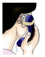
b. Add-on amplifier: This type of amplifier can be attached to the receiver end of the existing telephone. It can be removed from the telephone. The biggest advantage of this amplifier is that it can be used with different phones. The user may even carry the add-on amplifier around and use it when he/she uses public/other phones. These amplifiers are also cheaper and easy-to-use. However, they may not work with all phones. Also, batteries need to be changed regularly.
