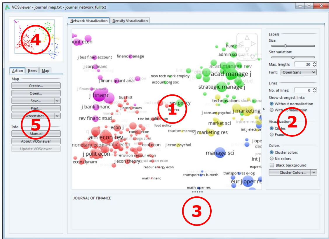
Figure 1. The main window of VOSviewer. The numbers indicate (1) the main panel, (2) the options panel, (3) the information panel, (4) the overview panel, and (5) the action panel.
